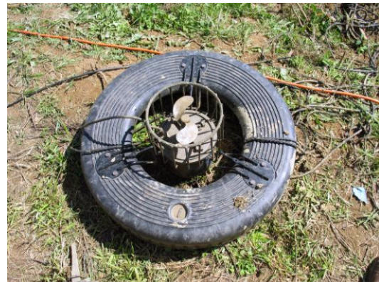
Vertical pump aerator with ring float
