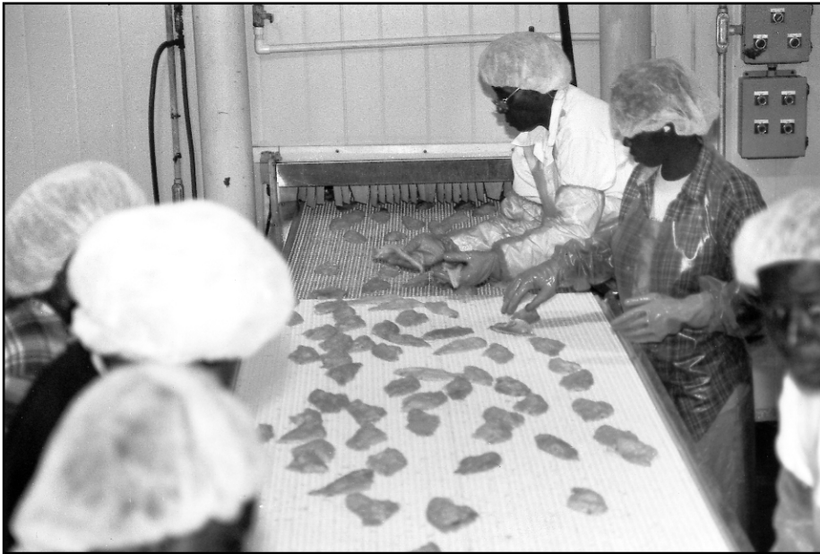
Figure 14. Fillets are individually quick frozen (IQF), glazed and packaged.
