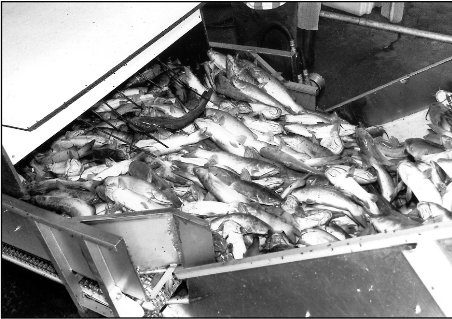
Figure 4. Fish are electrically stunned before processing.
