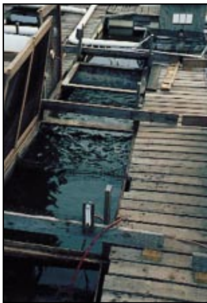
Figure 1. IPR with dock—note blower housing and air-manifold are at the forward end of the raceway.
