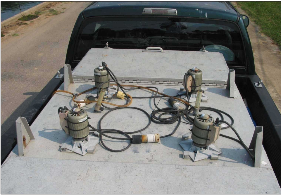
Figure 5. Agitators and electrical connections on an aluminum pickup truck tank.
