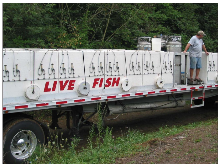
Figure 2. Semi truck-trailer carrying fiberglass transport tanks with round drain plugs and liquid oxygen dewars.
