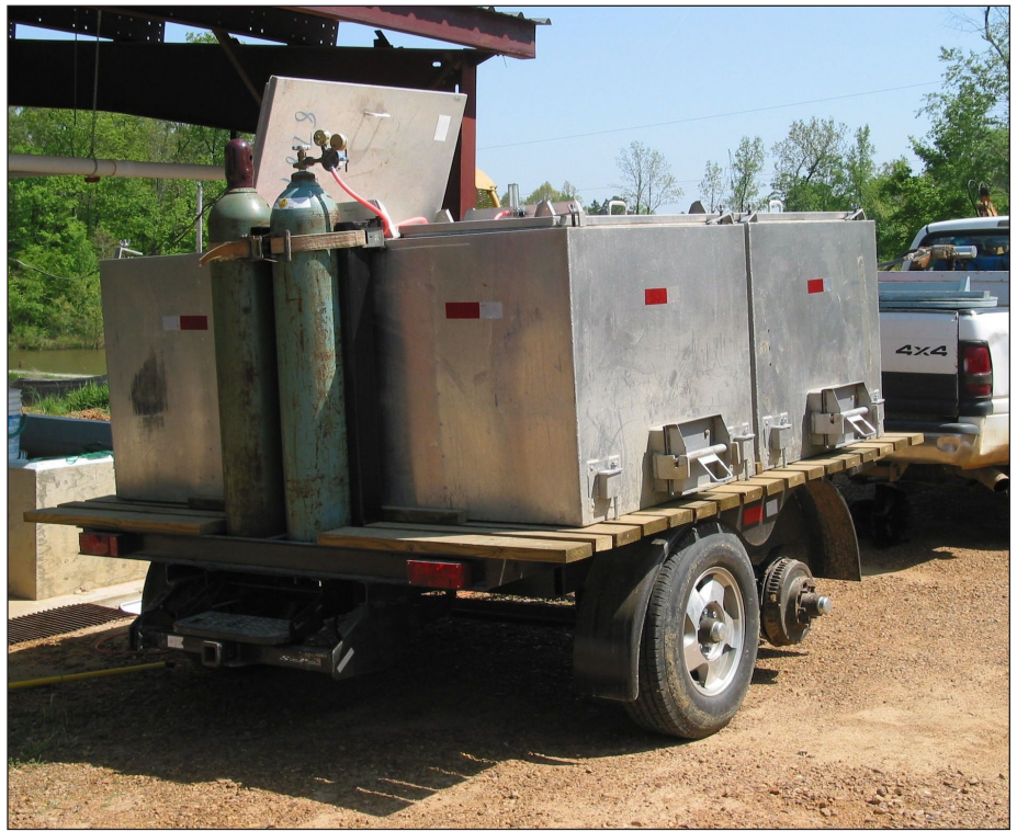
Figure 7. Compressed oxygen gas cylinders mounted on a trailer.
