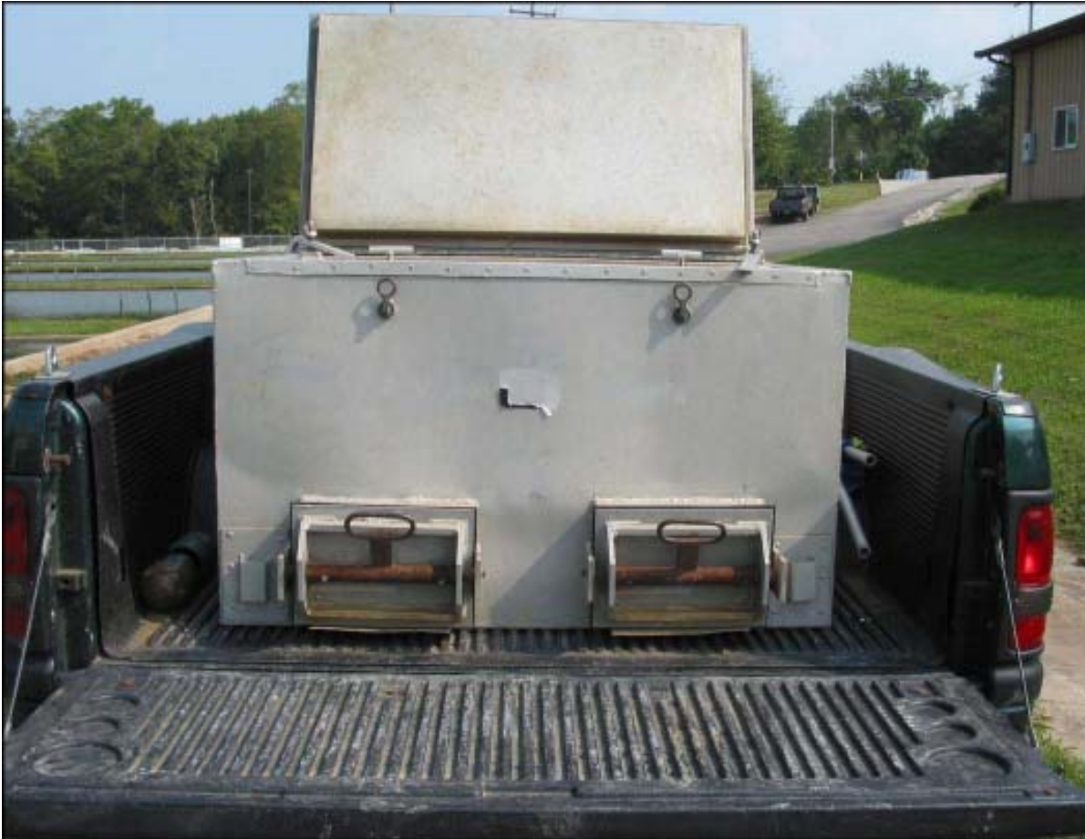
Figure 5. Small aluminum pickup truck transport tank
