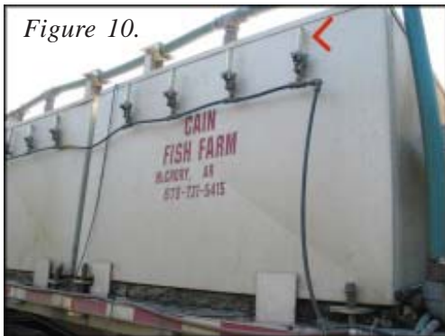
Liquid O 2 line with O 2 flow meters
