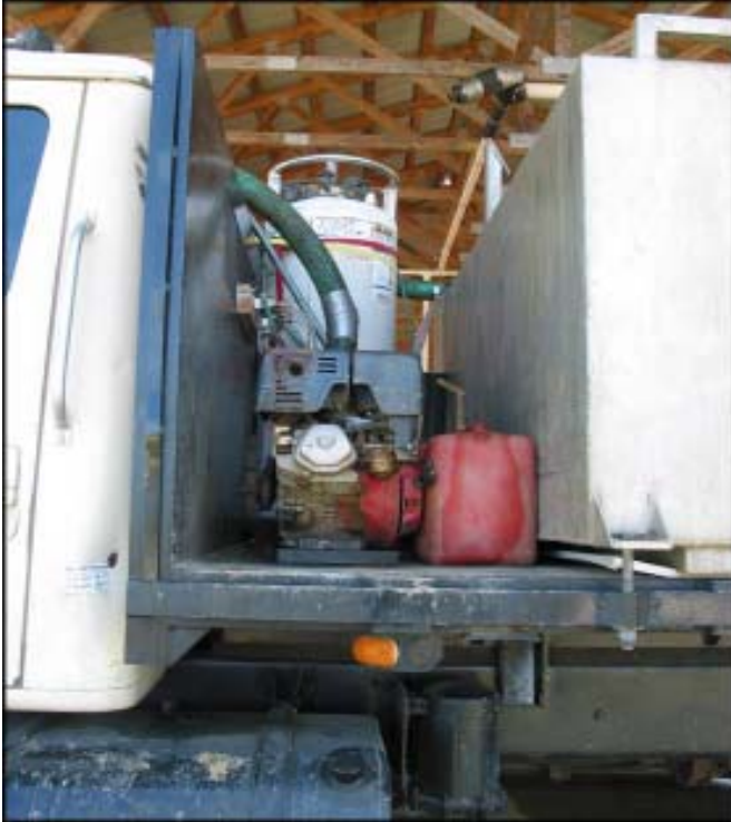
Truck equipped with air blower and liquid oxygen
