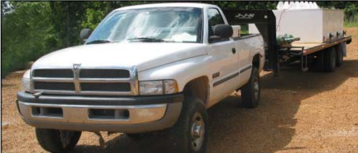
A pickup with gooseneck trailer can haul a number of fish tanks.
