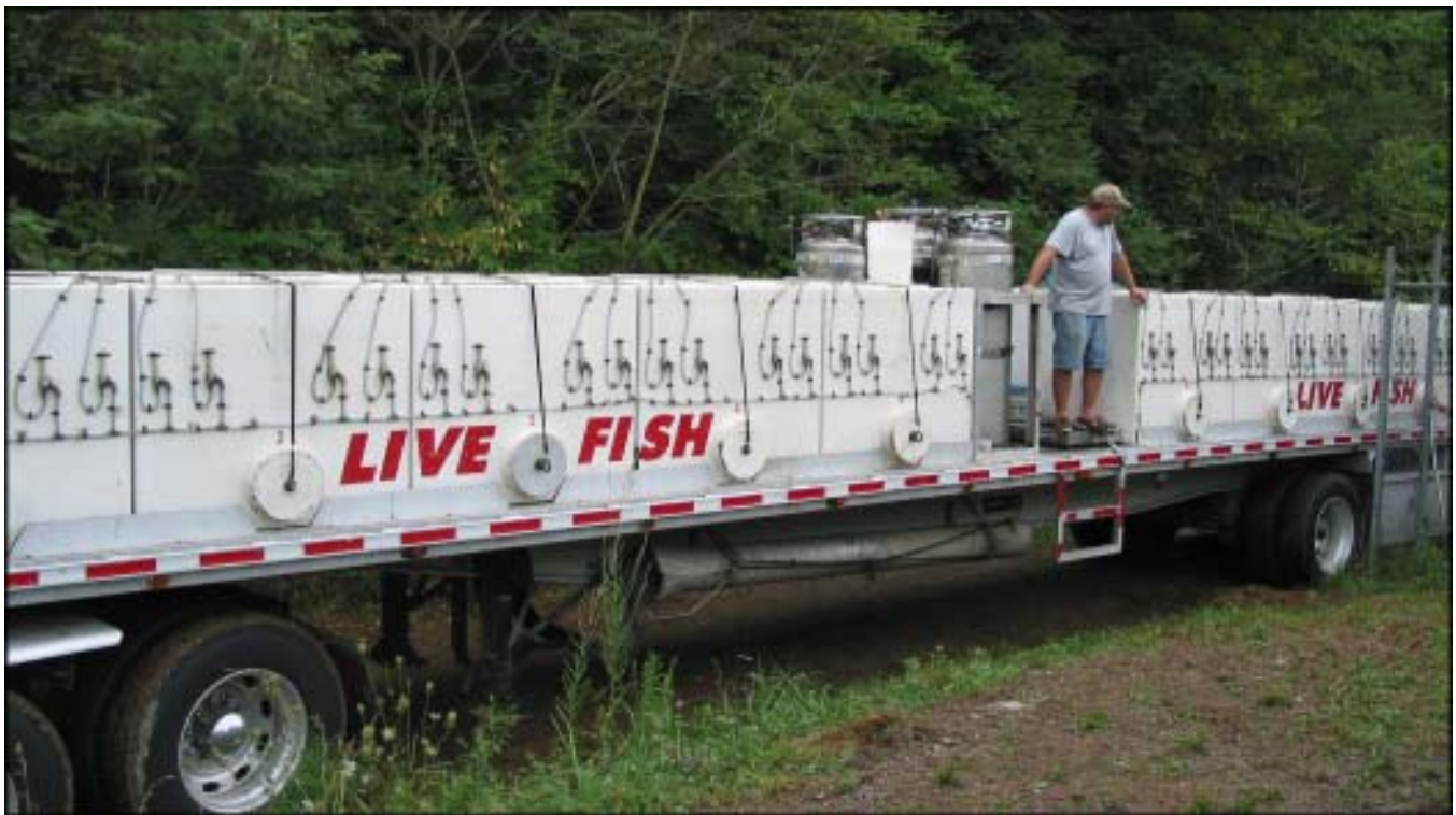
Figure 6. Large fiberglass tanks installed on a flatbed trailer
