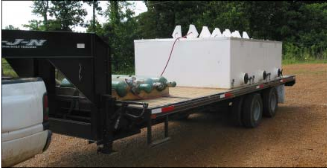
Gooseneck trailer with tanks and compressed O 2 bottles
